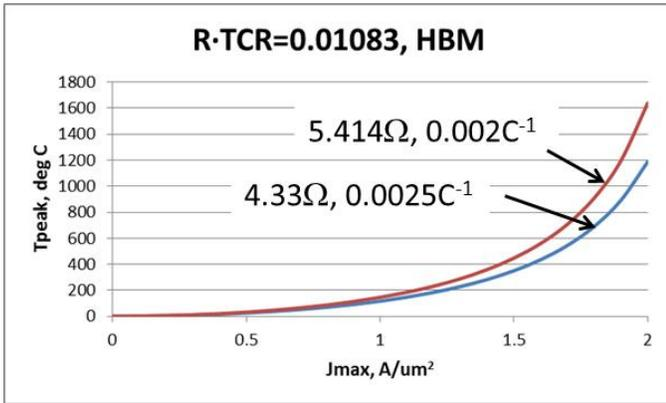
Figure 10.  $T_{max}$  vs.  $J_{max}$  for HBM from Eq. (3); constants from Eqs. (6).
