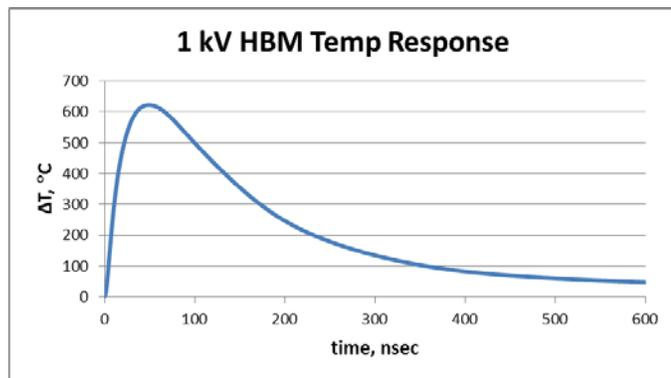
Figure 6. Temperature waveform of a typical mid-level metal test pattern with  $0.5 \mu\text{m}^2$  cross-section, subjected to a 1kV HBM pulse.
