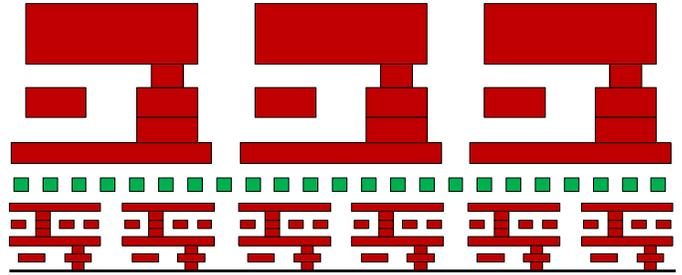
Figure 1. Cross-sectional view of heated lines (middle) surrounded by oxide and “dummy” metal and via layers above and below.
