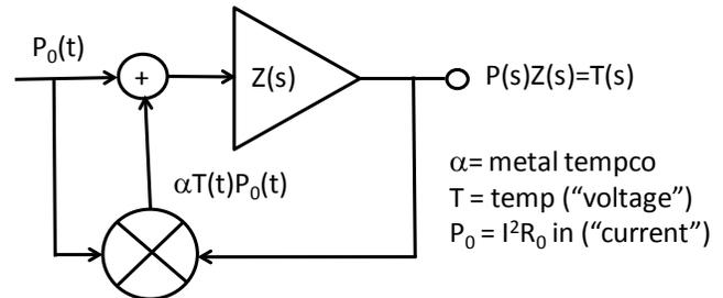
Figure 2. Feedback model of interconnect metal heating, as in [1].
