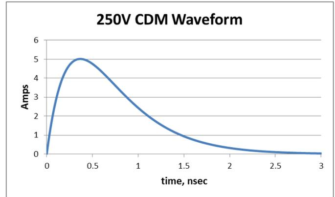
Figure 7. CDM current waveform at 250V charging voltage.
