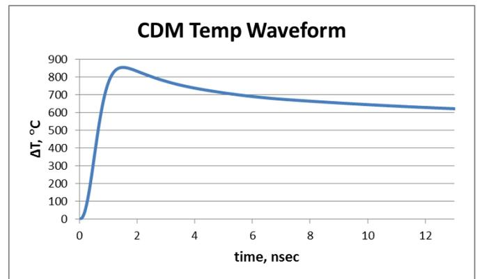
Figure 8. CDM temperature waveform example at 250V, for an upper-level metal test pattern.
