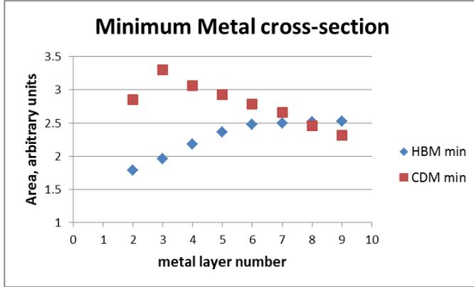
Figure 13. General trend of minimum cross-sectional area (in arbitrary units) as a function of metal layer for HBM (1kV) or CDM (250V) peak temperature to be limited to 1050°C.
