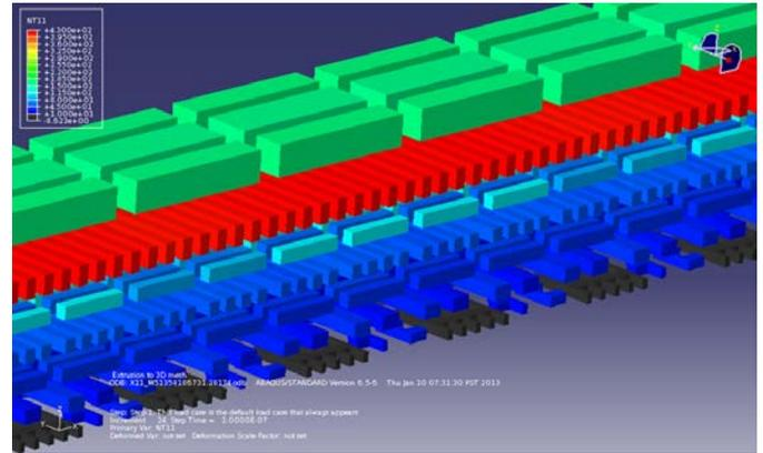
Figure 4. Typical FEM result after 200 nsec for a power step input to wide metal lines (red) as in [1]. Upper metal is thermally floating.
