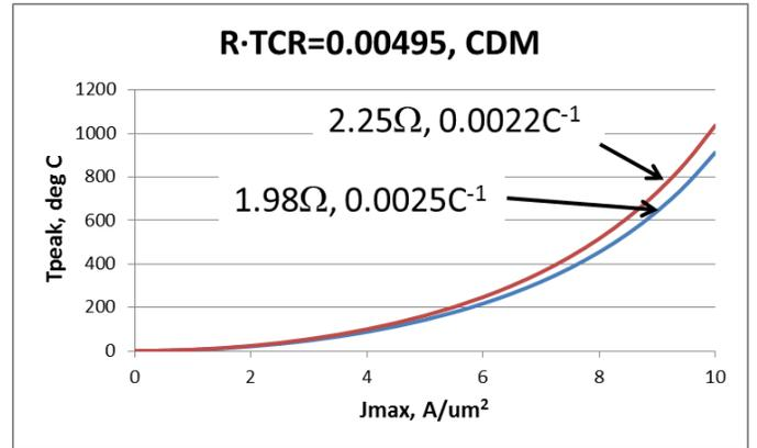
Figure 12.  $T_{max}$  vs.  $J_{max}$  for CDM from Eq. (3); constants from Eqs. (7).
