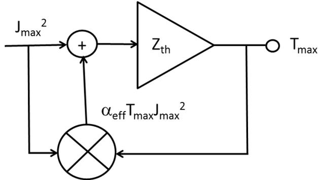
Figure 3. Simplified feedback model for  $T_{max}$  during ESD.
