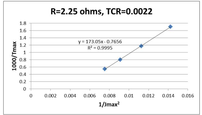
Figure 11. Inverse quantity plot for CDM, 200-275V. R is resistance of an upper level metal test pattern at  $T_0$ ,  $0.5 \mu\text{m}^2$  cross-section.
