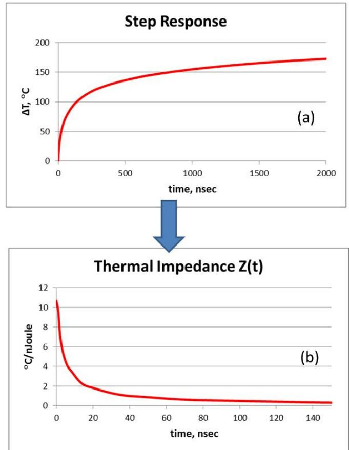
Figure 5. (a) Temperature increase of a metal test pattern in response to uniform power input, 0.6575W in this case. (b) Derived impulse response.
