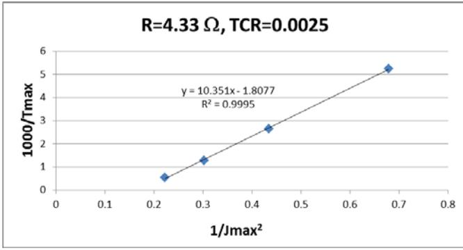
Figure 9. Inverse quantity plot for HBM, 0.8-1.4kV. R is resistance of a mid-level metal test pattern at  $T_0$ ,  $0.5 \mu\text{m}^2$  cross-section.
