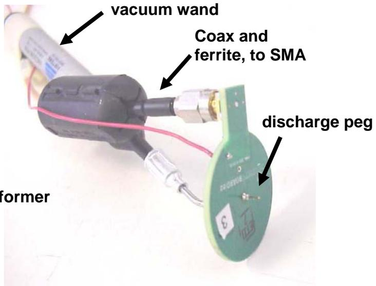
Figure 3. Instrument from side with discharge peg.
