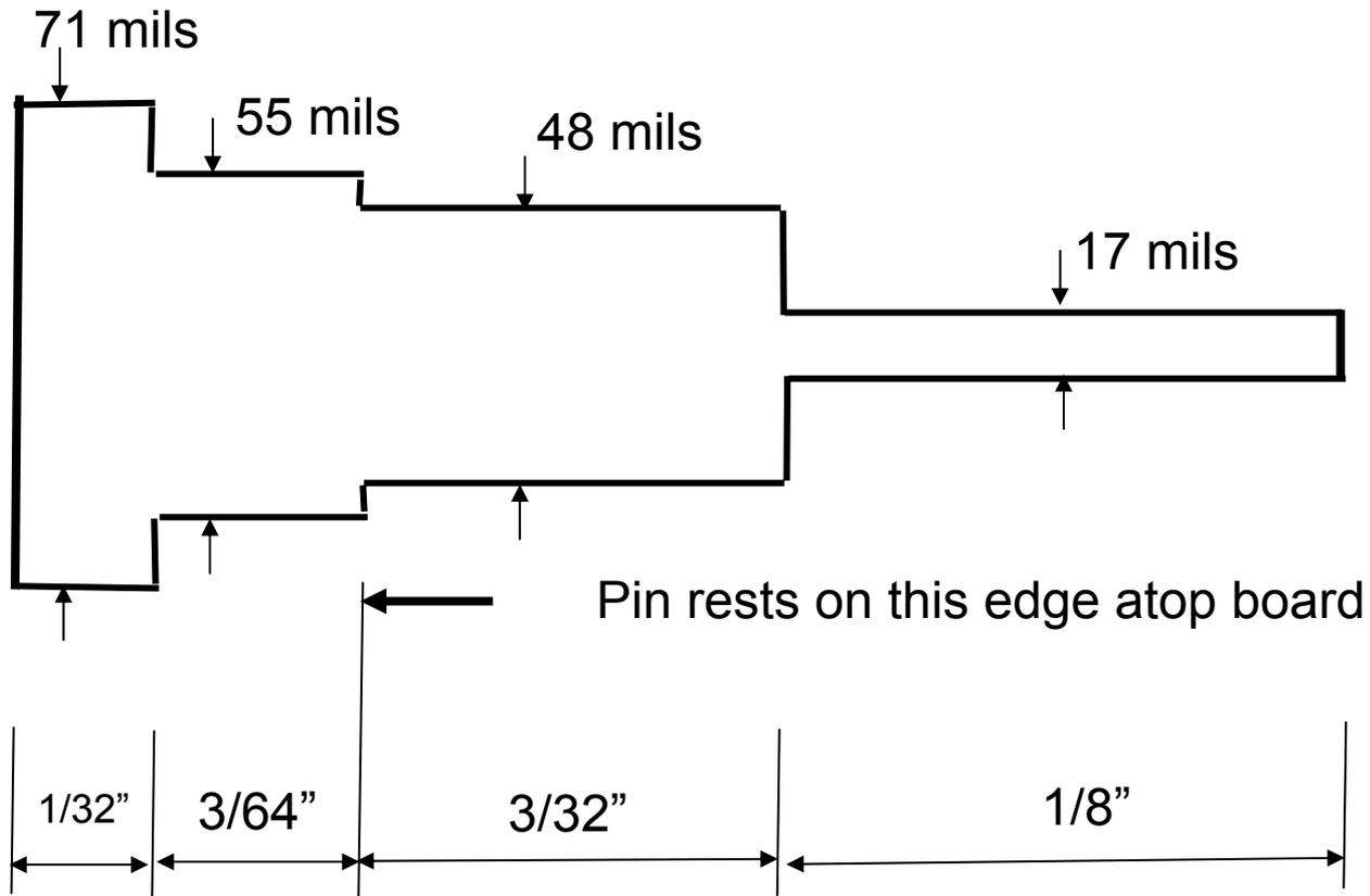
**Should be around 3-3.5 nH to “shielded” line on board**
