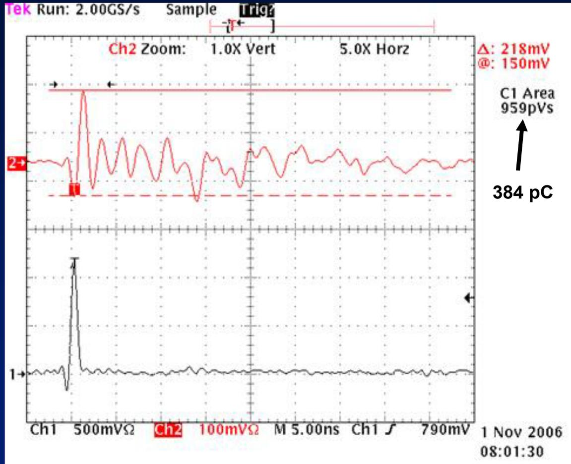
100V zap on copper board, ~30 cm; 568 mV/nC
