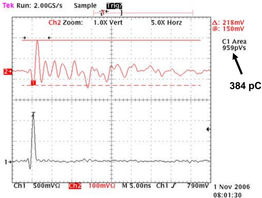
Figure 4. Scope traces; Ch. 1 discharge from board at 100V, Ch. 2 from antenna.
