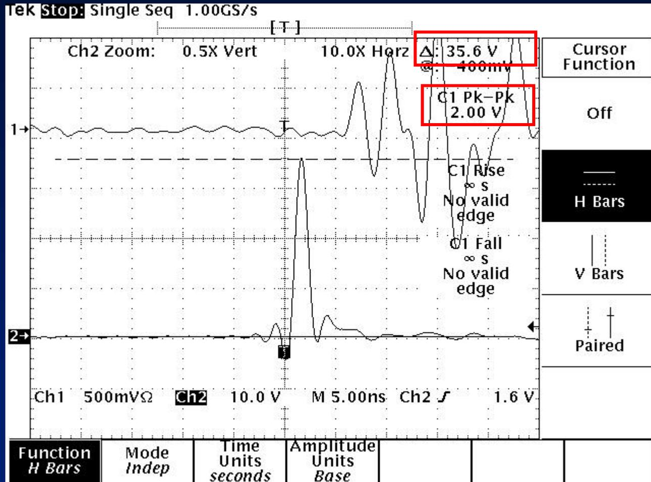
Ch2 base (2.6 nsec here) x height ÷ 50 ohms gives charge packet
