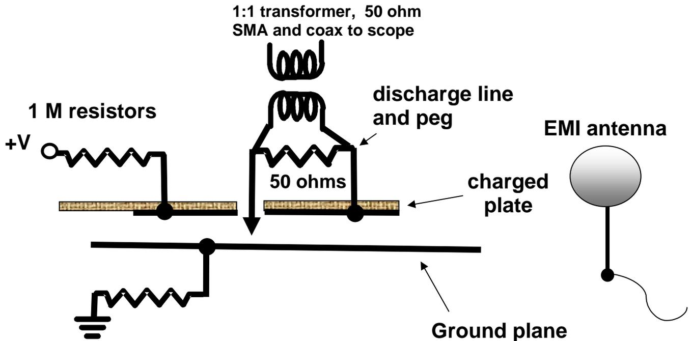
Figure 1. Schematic diagram of discharge instrument, plus EMI antenna.
