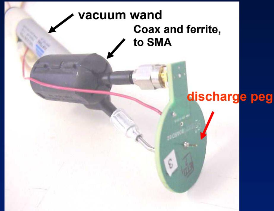
**1.25" diameter circuit board, plus tab for SMA connector**
