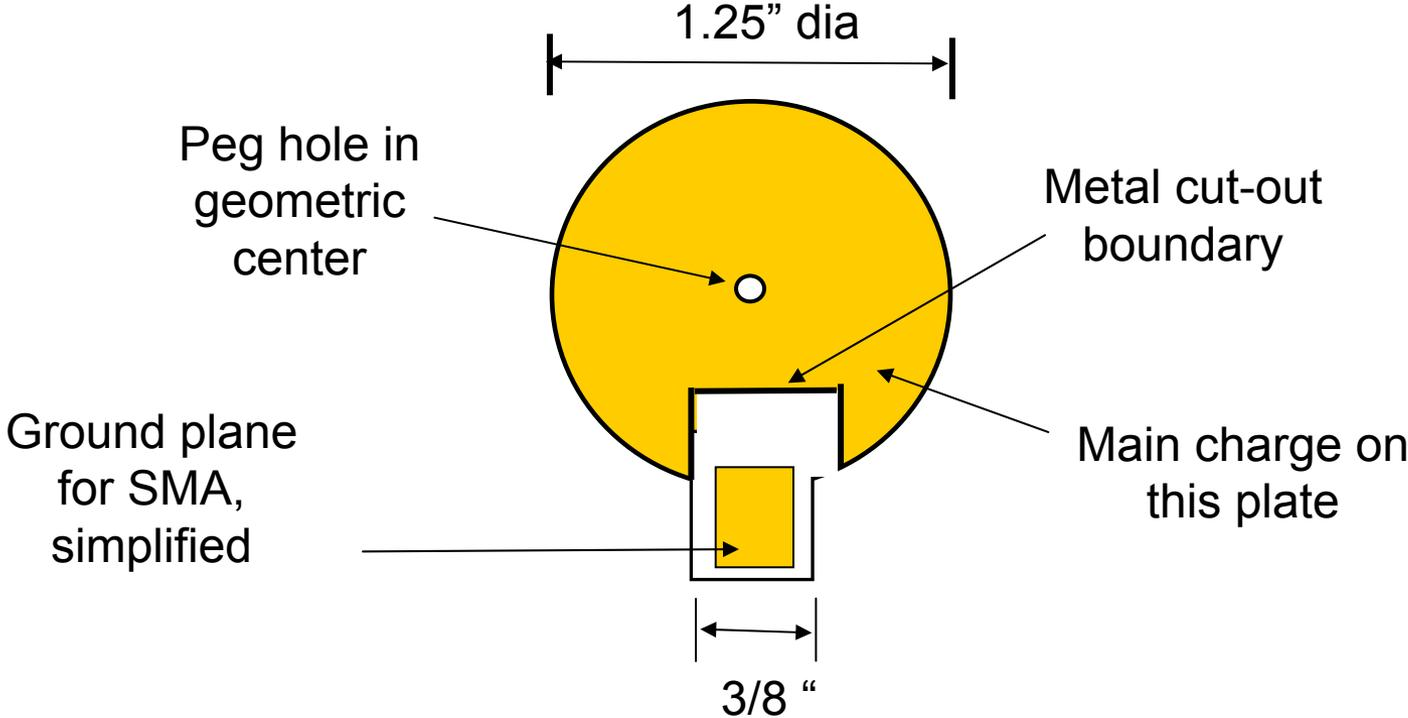
Metal cut-out avoids parasitic capacitance to xformer and SMA feed
