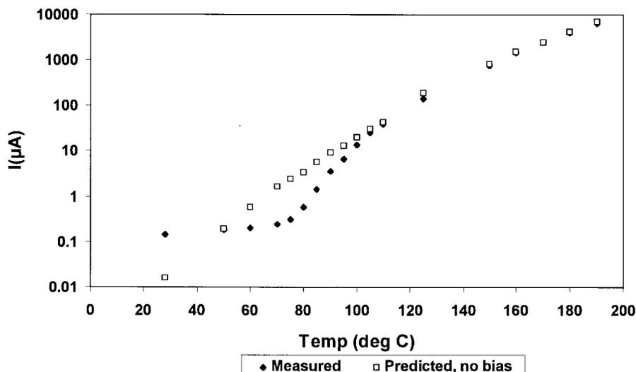
Fig. 11. Six-stage p-channel cladded diode string  $I$  versus  $T$  for Fig. 12, compared with unbiased current as calculated from individual cell data.
