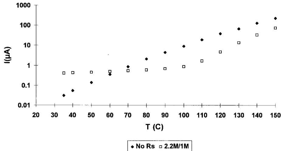
Fig. 9. Measured leakage for 3.0–5.5 V six-stage cladded diode string, with discrete resistors as in Fig. 8. Values were chosen to allow low leakage up to 100 °C.
