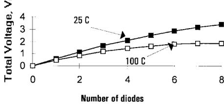
Fig. 6. Diode string turn-on voltage for two temperatures for  $\beta = 6$ .
