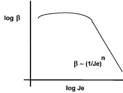
Fig. 7. Log of current gain versus log of emitter current density for a typical diode string p-n-p transistor, allowing simplified modeling of the diode string performance. The coefficient  $n$  is measured for each process.
