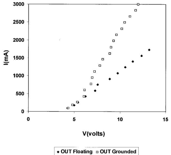
Fig. 17. Pulsed  $I$ - $V$  curves for six-diode cantilevered string in process  $P_2$  (see Table I); OUT floating includes the required termination circuit, and OUT grounded indicates how much voltage develops across that circuit as well as the six-diode  $I$ - $V$  relation.
