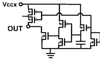
Fig. 18. n-FET termination for cantilever clamp. The diode bias network is also shown.
