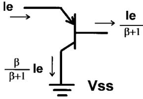
Fig. 5. Current gain effects in the p-n-p bipolar transistor formed by a diode stage.
