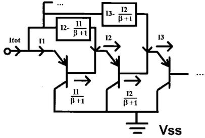
Fig. 20. Currents in p-n-p diode strings with bias.
