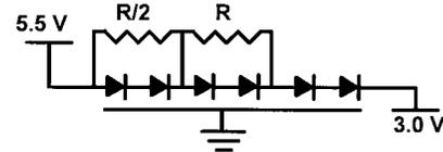
Fig. 8. Bias network for a six-diode mixed power supply clamping string, designed to maximize the temperature at which leakage current of  $\Delta V/R = 2.5/R$  flows, while using minimum total resistance.
