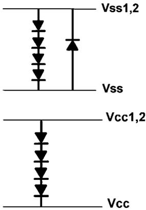
Fig. 2. Typical diode strings between peripheral and core power supplies. Note the bidirectionality of the  $V_{ss1,2}$ - $V_{ss}$  clamps, owing to the output NMOS transistor sources.
