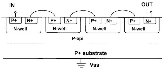
Fig. 3. Cross-sectional view of four-stage diode string in p-substrate CMOS.
