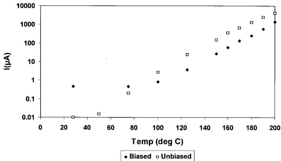
Fig. 14.  $I$  versus  $T$  for eight-stage diode string as in Fig. 13, shown with and without booster network enabled. This circuit is intended as a  $V_{CC}$  clamp for a low-voltage process.
