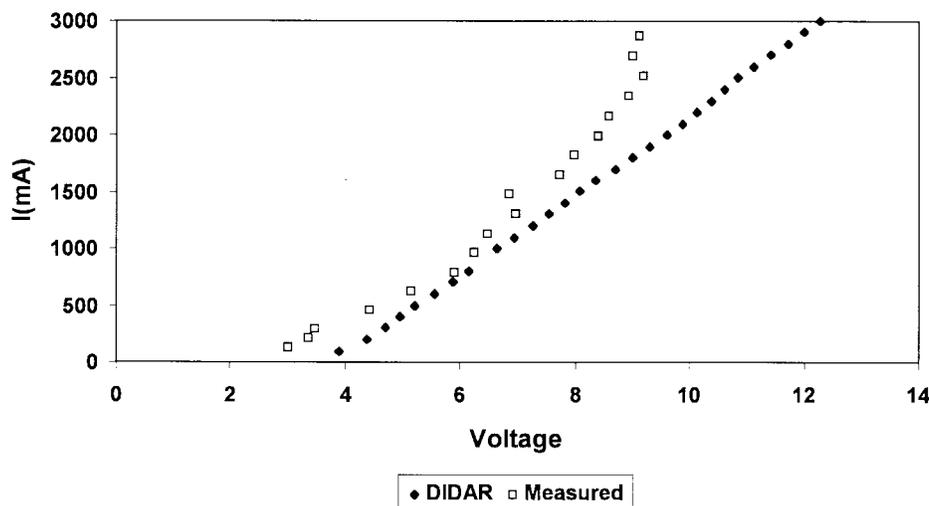
Fig. 19. Measured and modeled pulsed  $I$ - $V$  curves for cantilever clamp in the process  $P_1$ .
