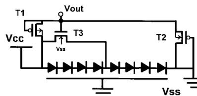
Fig. 13. Boosted diode string as achieved with buffered voltage divider in the form of long-channel leaker pair  $T_1$  and  $T_2$ , and source follower  $T_3$ , supplying extra bias current to the middle of a long diode chain only when needed.
