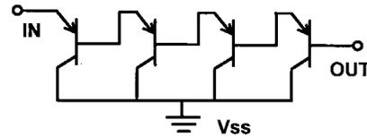
Fig. 4. Four-stage diode string of Fig. 3, seen as a chain of p-n-p transistors.
