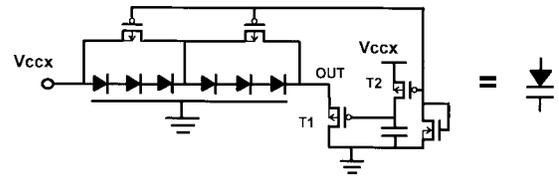
Fig. 16. Six-stage cantilevered diode string with resistive bias network and termination circuit. The suggested circuit symbol could apply to any cantilever clamp network.
