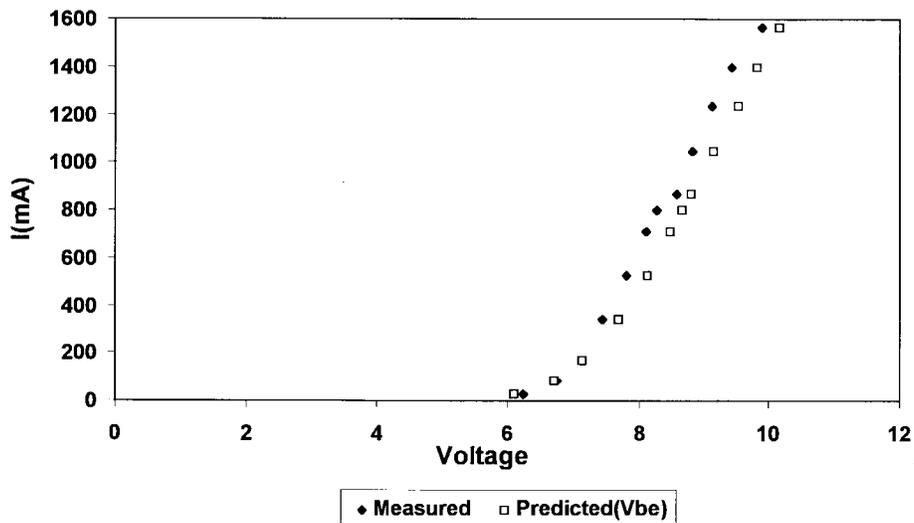
Fig. 15. Pulsed  $I$ - $V$  measurements for boosted eight-stage clamp, and comparison with model prediction.
