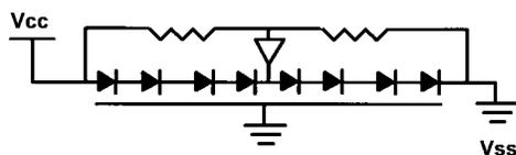
Fig. 12. Use of a buffered voltage divider to supply extra bias current to the middle of a long diode chain.
