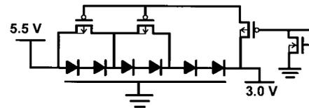
Fig. 10. Cladded bias network implemented in p-channel FET's for a six-diode mixed power supply clamping string, intended for a process limited to 3.6 V across gate oxides.
