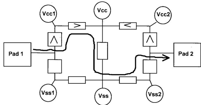
Fig. 1. Example of preferred ESD current path from one pad to another, showing passage through I/O circuits, and core power supply clamps for a positive zap. Boxes with arrows indicate strongly directional devices; others are bidirectional. It is also clear how the current path could terminate at any one of the power supply lines by passing through the elements shown.
