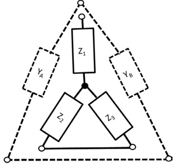
Figure 2:  $Z_1$ - $Z_2$ - $Z_3$  “Y” network of Fig. 1 converts to  $Y_A$ - $Y_B$  “delta” network such that admittances add due to the  $Z_2$ - $Z_3$  short.
