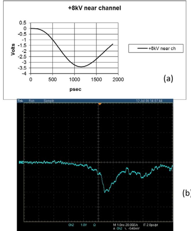
Figure 12: (a) Calculated near end signal for +8kV IEC pulse applied at point A. (b) Measured near end signal. Scope set at 1V/div, 1 nsec/div.
