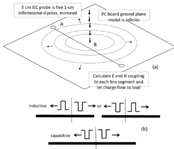
Figure 10: (a) Geometric scheme for calculation of IEC gun pulse to ground; Fig. 9 setup would have pulse source at point A. (b) Line segment charge flow as caused by H (inductive) or E (capacitive) fields.
