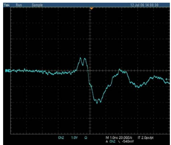
Figure 13: Measured signal from +8kV IEC pulse applied at point B, middle of board. Scope set at 1V/div, 1 nsec/div.
