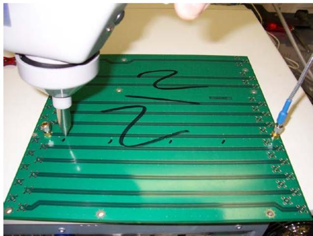
Figure 9: Printed circuit board with 50-ohm trace, terminated at each end. IEC gun pulse can be applied to exposed ground anywhere near the trace or at step displacements.
