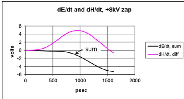
Figure 14: Calculated field derivatives from +8kV IEC pulse applied at point A, resulting from sum and difference currents on a 20 cm line. The effective  $dH/dt$  reaches zero a reasonable propagation time after the IEC pulse peak current.
