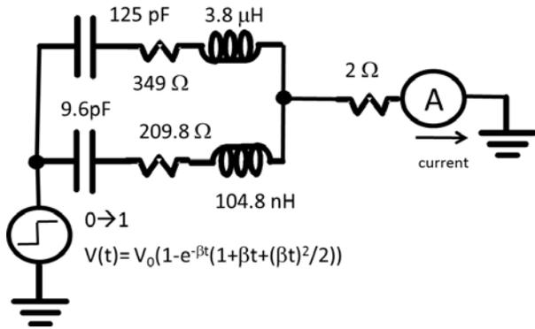
Figure 4: Model from [7], inspired by fitting double-pole functions ( $i(t) = Ate^{-\alpha t}$ ) to the IEC waveform.
