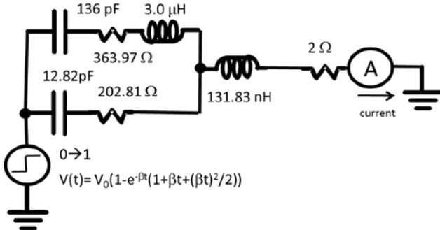
Figure 1: Circuit model for “nominal” waveform, from [5]. Here we use a “soft” step function,  $\beta=15$  GHz.
