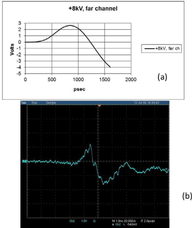
Figure 11: (a) Calculated far end signal for +8kV IEC pulse applied at point A. (b) Measured far end signal. Scope set at 1V/div, 1 nsec/div.
