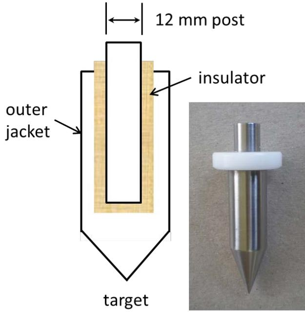
Figure 6: Schematic drawing, and inset photo, of capacitive coupling tool for an IEC pulser. Metal probes are separated by Delrin® dielectric, and series capacitance of 25 pF is measured.
