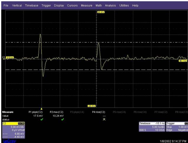
Figure 13. Monocycle pulse (left, 175 mV= $V_{p-p}$ ) and its reflection from ESD event detector (right, 112 mV) after transit of 150 cm cable (15 nsec). Here the cable and event detector were on Port 2 and Port 3, 20 dB down, was routed to the oscilloscope.
