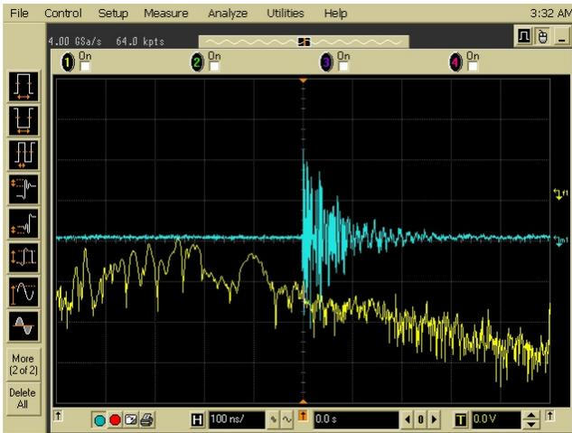
Figure 10. Waveform (100 ns/div) and spectrum (200 MHz/div; 1GHz at middle, 20 db/div) for ns-CDM machine (Fig. 8) zap of 500 V, 2.5 nC charge packet, Vp-p of 882mV, ball antenna 30 cm (12") above aperture.
