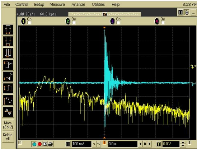
Figure 9. Waveform (100 ns/div) and spectrum (200 MHz/div; 1GHz at middle, 20 db/div) for ns-CDM machine (Fig. 8) zap of 500 V, 2.5 nC charge packet, Vp-p of 3.5V, ball antenna 15 cm (6") above aperture.
