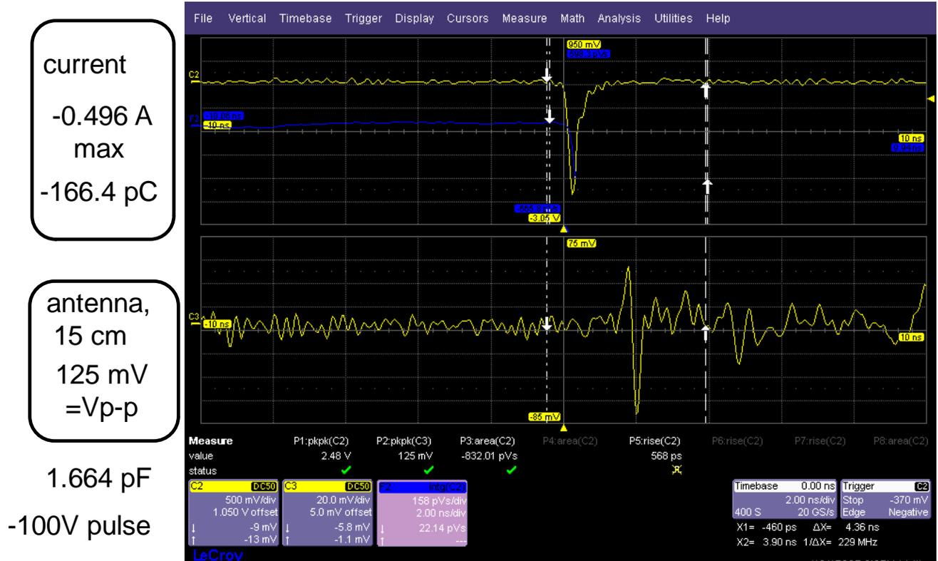
Fig. 3. Measured current (top) and antenna response (bottom) to E-field at 15 cm, using artificial CDM source; 2 nsec/division, 3 GHz scope. Setup as in Fig. 1, current polarity negative. Integrated current gives -166.4 pC of charge; 10x attenuation used.
