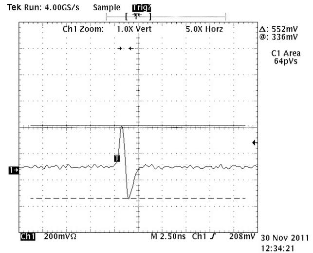
Fig. 5. Monocycle pulse output [3, 4].  $V_{p-p}$ =552 mV after 10X attenuation. 1 GHz scope, 2.5 nsec/division.
