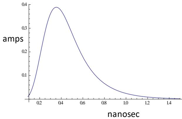
Fig. 4a. CDM current pulse that approximates current pulse measured in Fig. 3. 1.5 nsec full scale.
