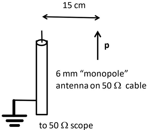
Fig. 1. Experimental arrangement of CDM electric dipole initial source  $\mathbf{p}$  and 6 mm coaxial antenna.
