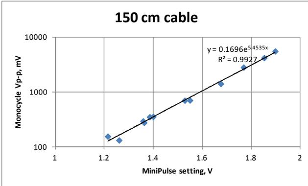
Fig. 6. Monocycle pulse peak-to-peak voltage ( $V_{p-p}$ ) magnitude vs. threshold setting of MiniPulse event detector, semi-log plot. Excellent agreement with exponential fit (422 mV/decade).
