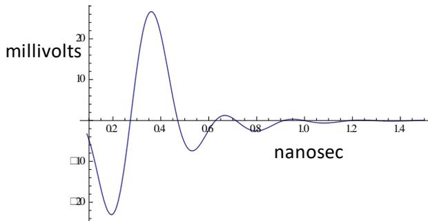
Fig. 4b. Calculated antenna response to E-field using current source of Fig. 4a. 15 cm from CDM source, 1.5 nsec full scale, 3 GHz scope filter. Alignment as in Fig. 1.
