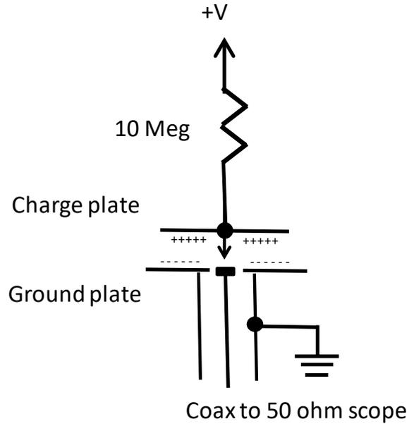
Fig. 2. CDM pulse generator. Charge plate probe hits pedestal and dipole collapses, with current pulse and dipole radiation.
