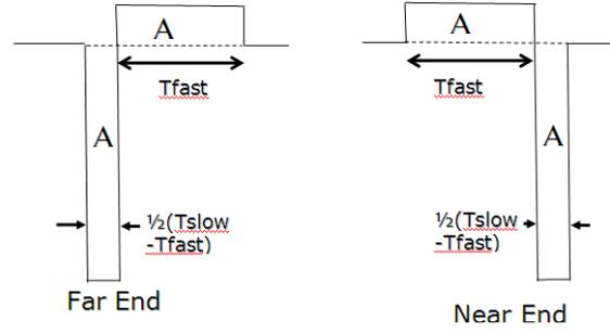
Fig. 13. Step response of far end and near end  $Z_{fe}$  loads on dielectric line for Case 3 as in Fig. 12. These are the L-pulses  $L_{fe}$  and  $L_{ne}$ .
