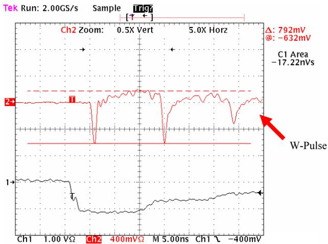
Fig. 4. W-pulse using Fig. 1 lab setup. Air line pulse shown in black, trace 1; ideally it would be a rectangular pulse imperfect Z-matching gives waveform shown and some multiple reflections. Even so, the first time step shows the W-pulse, trace 2 in red.
