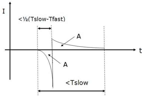
Fig. 14. Sketch of induced current response on data lines, resulting from a pulse as in Fig. 2 on the shield. With inductive coupling only, velocity contrast causes a large short negative pulse followed by a long positive pulse, thus a latchup hazard. The strong initial signal at the far end (shield touching ground, Fig. 2) induces current that flows smoothly on the dielectric line, giving the time-compressed short initial spike at the near end load, despite the weak E-field in that vicinity.
