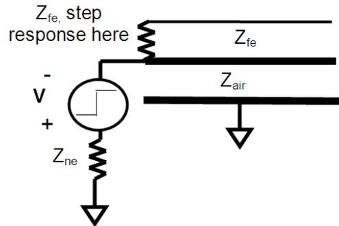
Fig. 10. Case 2 step response situation;  $Z_{air}=Z_{ne}$  and  $Z_{fe}$  match for eigenpulse. Pulse is applied to platform chassis at shield connection (near end), cable far end open. Current is induced on platform data lines and into platform load  $Z_{fe}$ .
