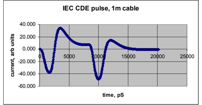
Fig. 9. Convolution result (Eq. 1) for Case 1A, IEC pulse applied to FE open end of cable shield and signal at NE platform data lines shown. 1 meter cable;  $v/c=1$  for air line and 0.67 for dielectric line. The main convolution effect is bipolar pulse pairs, produced as each spike doublet (Fig. 8) sweeps across the leading section of the IEC pulse. For 1m,  $T_{fast}=6.7$  nS and  $T_{slow}=10$  nS.
