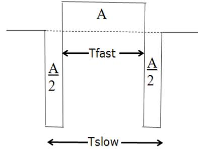
Fig. 5. Ideal Case 1 W-pulse for Z-match at far end (FE) on air line and Z-match on near end (NE, platform) cable line, other connections open (Fig. 3). Data lines at NE feel this. Areas balance due to inductive-only coupling.  $T_{fast}$  is round trip delay of fast (air) line,  $T_{slow}$  is round trip delay of slow (dielectric) line. Sharp spikes are due to the pileup of forward coupled waves.
