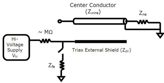
Fig. 3. Lab setup (from [1]) for creating the Case 1 W-pulse using triaxial cable. Outer line has constant impedance and simulates real world air line.
