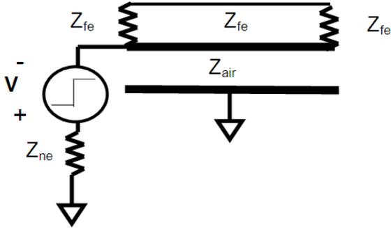
Fig. 12. Case 3 step response situation;  $Z_{air}=Z_{ne}$  and  $Z_{fe}$  matched at both ends of dielectric line for eigenpulse. Pulse is applied to platform chassis at shield connection (near end). Current is induced on platform data lines and into platform loads  $Z_{fe}$  but the pulses differ due to the step being at the near end.
