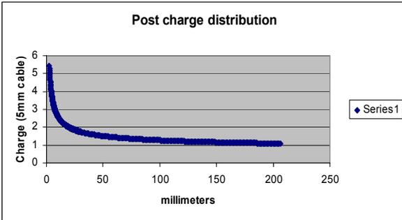
Fig. 2. Log-tapered charge distribution on a vertical shield or post of  $2a=5$  mm diameter, held at a constant potential perpendicular to a ground plane as in Fig. 1. With the height axis converted to time, this also generally describes the current pulse at the spark when the shield touches ground, and it describes the declining size of the current step with height as the hemispherical wave propagates upward.
