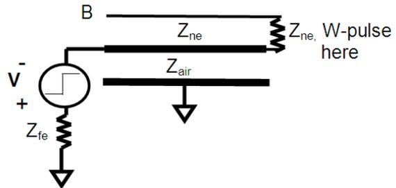
Fig. 7. Step response view of Case 1, W-pulse, felt at data lines on  $Z_{ne}$ .  $Z_{air}$  matches to  $Z_{fe}$  for eigenpulse, dielectric line matched at NE and open at point B. For the initially charged  $Z_{air}$  as in Fig. 3, superimpose this step with the initial +V on  $Z_{air}$  and you have W-pulse on  $Z_{ne}$  and square pulse on  $Z_{fe}$ , identical to Fig. 3.
