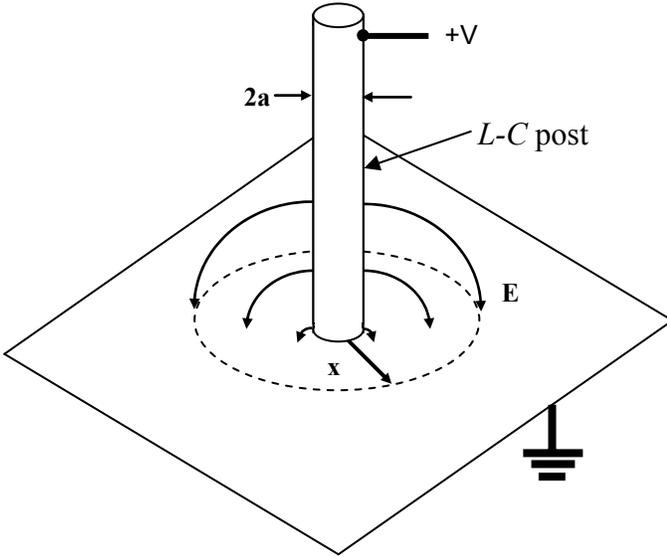
Fig. 1. Cable shield or wire as  $L-C$  post, with its electric field before discharge, as in [2].
